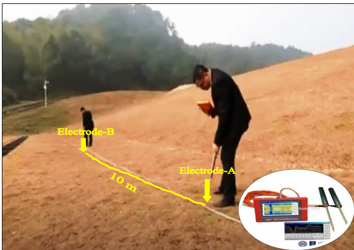
Figure-2: Showing the field procedure of PQWT Groundwater Survey (GWS)
